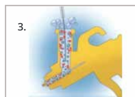
3. Next air is fed through another hose into the colour channel of the cleaning fluid. Micro-foam develops, which removes varnish and residues.
