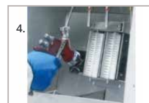
4. For cleaning the air cap piece there is a cleaning brush in the gun center. The varnish remains and the cleaner is disposed of and gathered in a blow-out opening.
