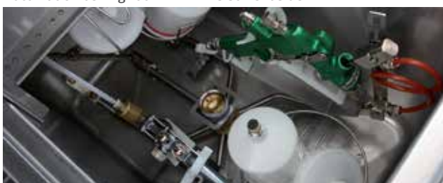
Automatic washing room LMW 115 solvent side
